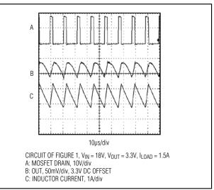
Figure 4. Continuous-Conduction Mode, Heavy-Load-Current Waveform
