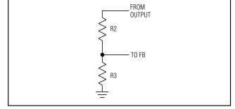
Figure 5. Adjustable-Output Operation Using the MAX1745
