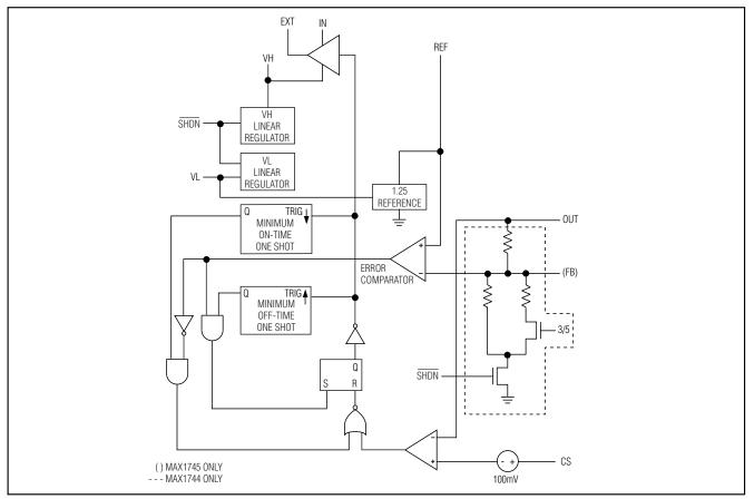
Figure 2. Simplified Functional Diagram
