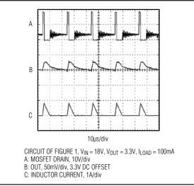
Figure 3. Discontinuous-Conduction Mode, Light-Load-Current Waveform
